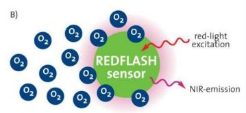
**Principle:** red light excited REDFLASH indicators show luminescence in the near infrared (NIR), which decreases with increasing oxygen (quenching effect).
